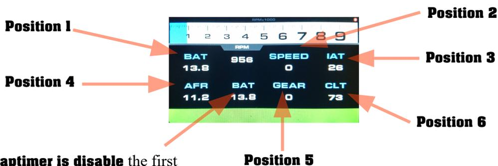
When **laptimer is disable** the first sensors with **no position and LOG active** will be displayed
